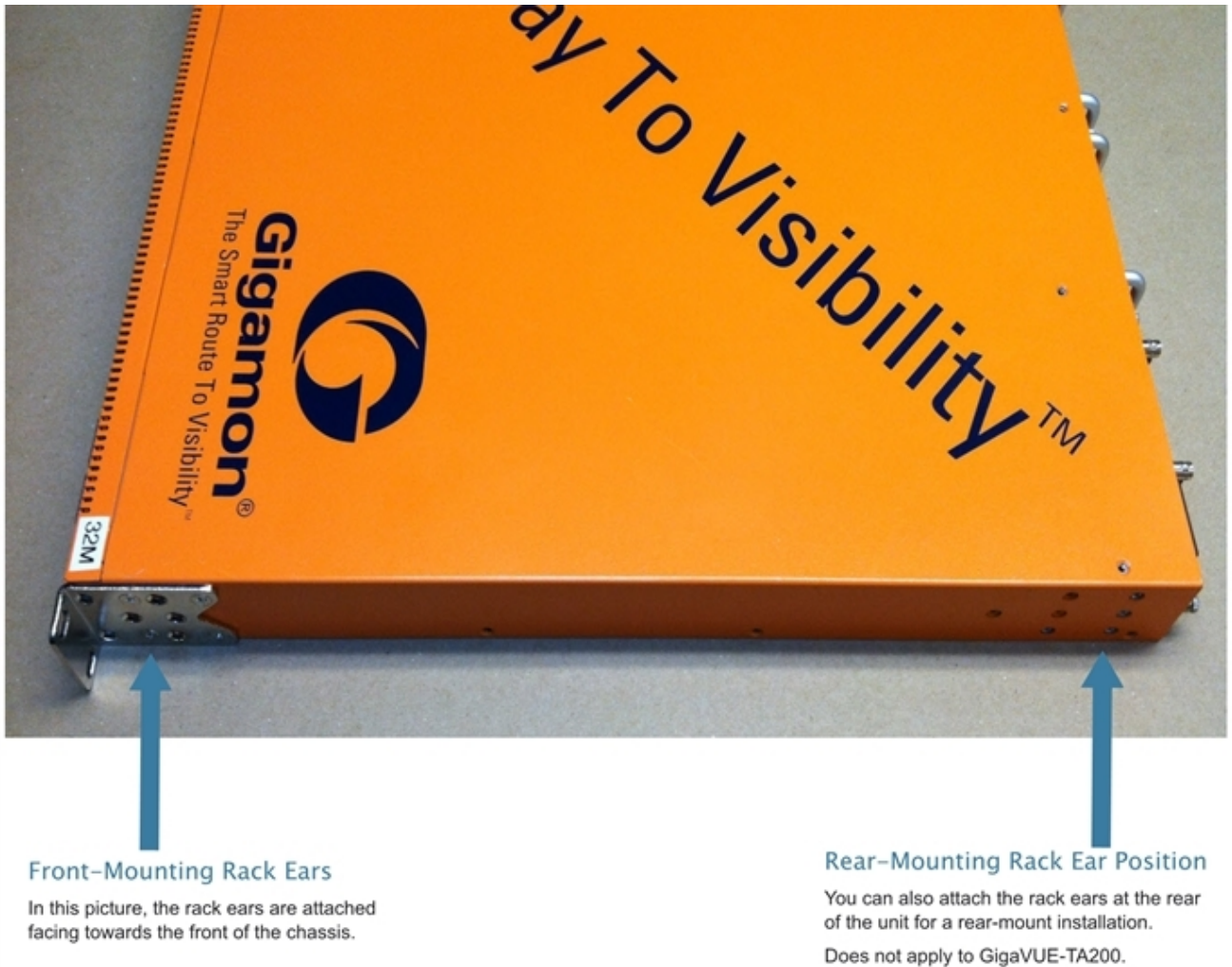
Figure 2 GigaVUE TA Series Traffic Aggregator Rack Ears in Front-Mount Position
