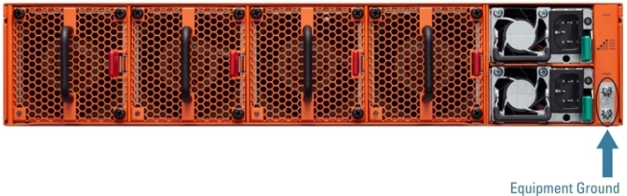
Figure 7 Ground Screws (GigaVUE TA Series-TA200 Shown)
